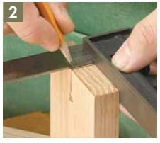
**Transfer the Mark** Now use a square to transfer the mark from the face to the end (or edge) of the workpiece. This line will be used to position the jig, as shown in *Fig. 3*.
