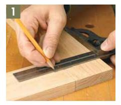
**Mark Centerlines** To lay out the mortises, dry assemble the pieces and mark centerlines across the joint line. Mark mating joints "A-A," "B-B," etc., so you can reassemble the pieces.
