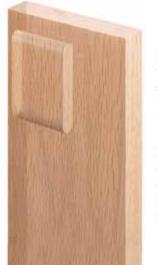
f you're planning to build a project with mortise and tenon joinery, you may want to consider this quick and easy variation instead — a mortise and tenon joint with a "loose" tenon. It has all the strength of a traditional mortise and tenon joint *without* the fussing around that's involved in getting a good fit.
